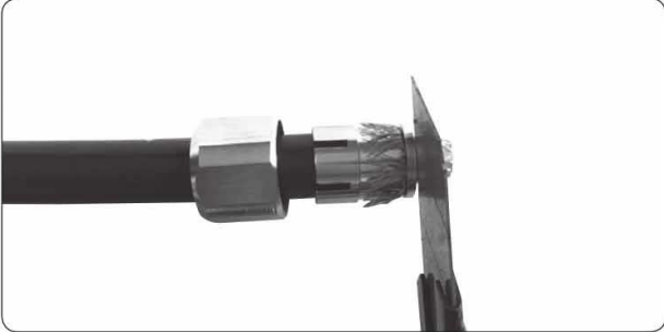
6. Cut off the aluminum foil and dielectric along the surface of the lining which will leave the pin exposed
