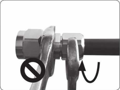
10. Tighten connector body firmly using the two wrenches as shown
